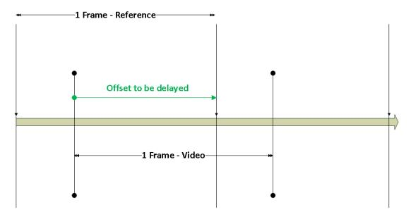
Figure 2: Offset of incoming video to reference signal
