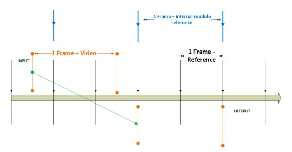
Figure 4: 720p50 ref with 1080i50 video - second possible internal clock interval
