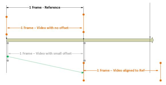
Figure 6: Synchronous video with small offset aligned
